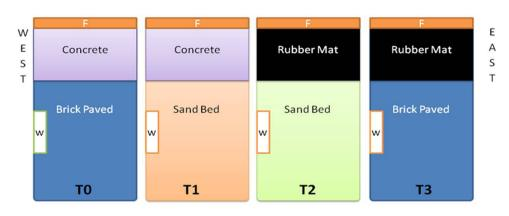
Figure 1. Schematic diagram of experimental shed with different flooring
