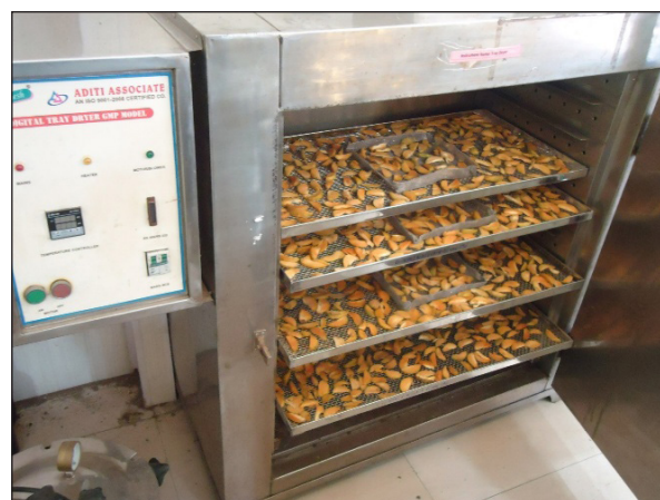
Fig. 1: Drying of sapota slices in tray dryer
