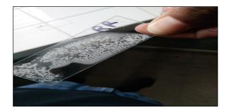
Fig. 1: Reaction of milk to White side test
