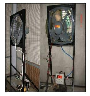
**Fig. 1:** Fan-Fogger system consisted of a blower with a copper ring having fine foggers (5 in no.) connected with a water tank through a high pressure pipe along the width wise of the pen
