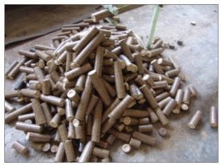
Fig 2: Briquettes of cotton and pigeon pea powder
