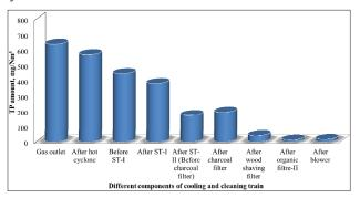
Fig. 6: Trend of TP observed in the cooling and cleaning train
