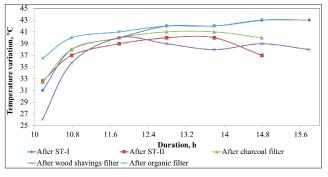
Fig 5: Temperature variation in the cooling and cleaning train
