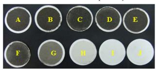
Fig. 7: Impression of TP on sampled papers collected at different points
