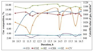
Fig 3: Variation in producer gas compositions and calorific value with duration
