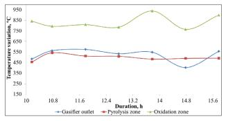
Fig. 4: Temperature variation in the reactor
