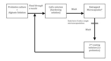
**Fig 2:** Flow diagram of extrusion process. The bacterial culture withalginate is dropped using a nozzle into hardening solution. Theproduced microcapsules are added into a second coating solution, if required. The process ends at \* if only a single encapsulation is required (Krasaekoopt *et al.*, 2003).
