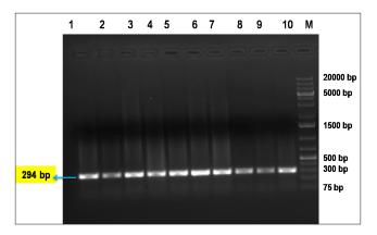
**Fig. 1:** PCR-RFLP electrophoresis pattern for Prolactin gene, Lane M: 100 –bp marker, Lane 1-8: undigested 294 bp fragment (Homozygous GG genotypes)
