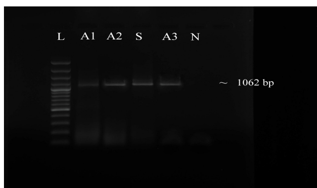
Fig. 3: PCR amplification of VP7 gene of bovine group A rotavirus with ~ 1062 bp amplicon. From left to right: Lane L - 1000 bp plus DNA ladder (Thermo scientific, 0.5 µg/ µl); Lane A1, A2, A3- Positive calf diarrhoea samples; Lane S - Positive control; Lane N -Negative control
