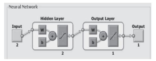
Figure 2 Two-layer feed-forward network
