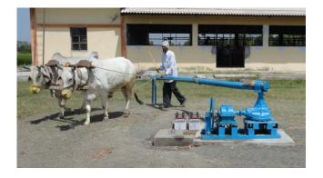
Fig. 1: Animal driven rotary mode system
