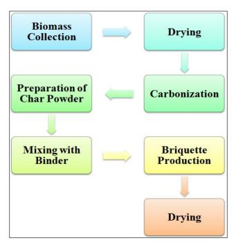
Fig. 2: Production process flow chart for briquette
