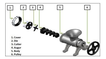
Fig. 3: Components of extruder type screw press briquetting machine
