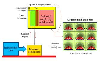
Fig. 1: Air tight multi-chamber temperature and RH control system
