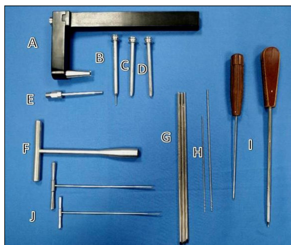
(A) Proximal and distal Aiming device; (B) Trocar; (C) Drill sleeve; (D) Drill sleeve; (E) Conical bolt; (F) Cannulated socket wrench; (G) Steinman pins trocar ended; (H) Long drill bits; (I) Extra long hexagonal screw drivers; (J) Extra long bone tap with T handle
